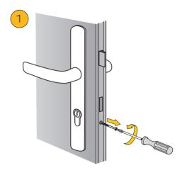
Remove (but keep safe) the screw to release the cylinder.
