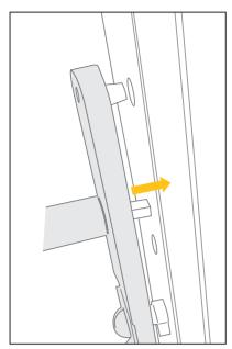
Use the protruding spindle as a guide to fit the internal Linus® L2 Backplate Handle to the inside of the door.
