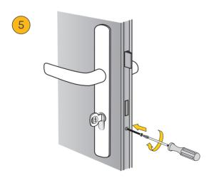
When aligned correctly the lock should operate smoothly and the screw can be replaced to secure the cylinder. If a smooth operation is not achieved, your Linus® Smart Lock L2 may not operate correctly.
