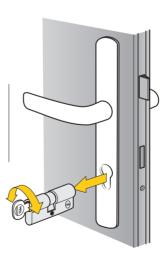
Remove the old cylinder. Use the key to align the cam (moving mid section) with the cylinder housing in order to push in/pull out the cylinder
