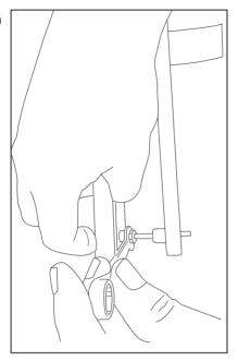
Once the correct fixing positions have been identified, tighten the screw bosses on the Linus® L2 Backplate Handle.
