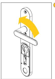
Turn the lever handle through 180 degrees to ensure the handle is in the correct orientation for your door.
