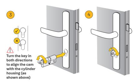
Insert the new cylinder with the cam aligned with the cylinder housing (as shown above).
