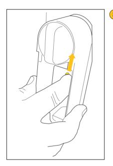
Slide the yellow switch inside the battery compartment upwards to firmly lock the Linus® L2 into position onto the Backplate Handle. Check it is securely attached by hand.
