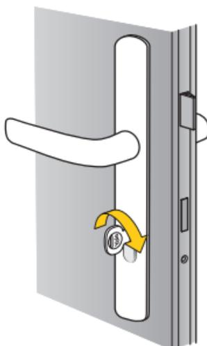
Check if the key turns and the lock operates correctly. If the key turns easily, the cam is aligned. If not, adjust cylinder position slightly and try again.
